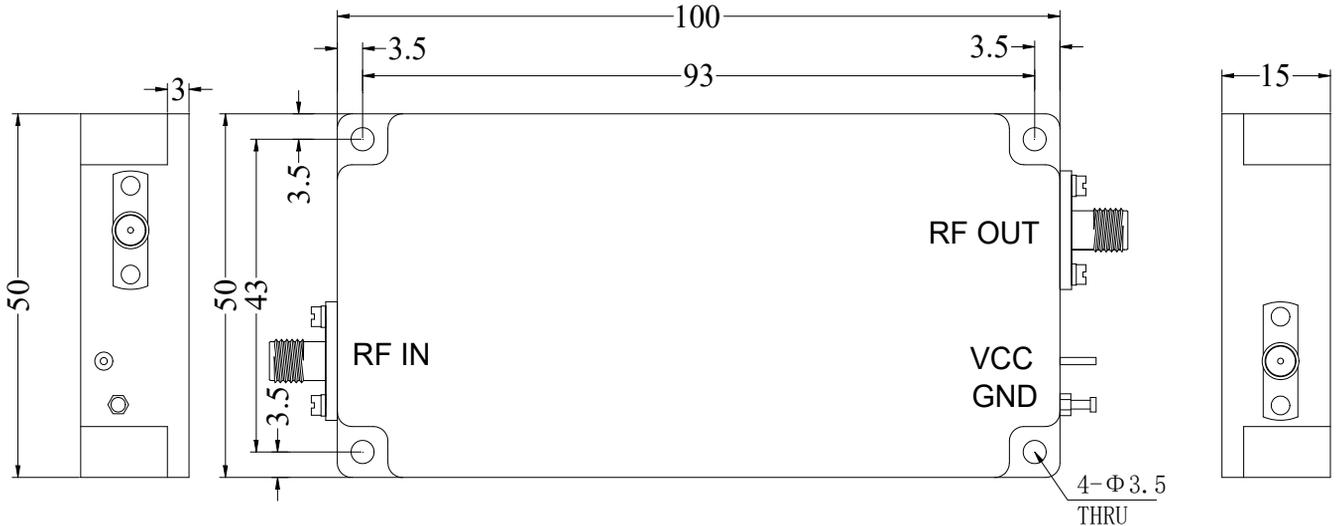
**\*\*\*Heat Sink Required During Operation**
